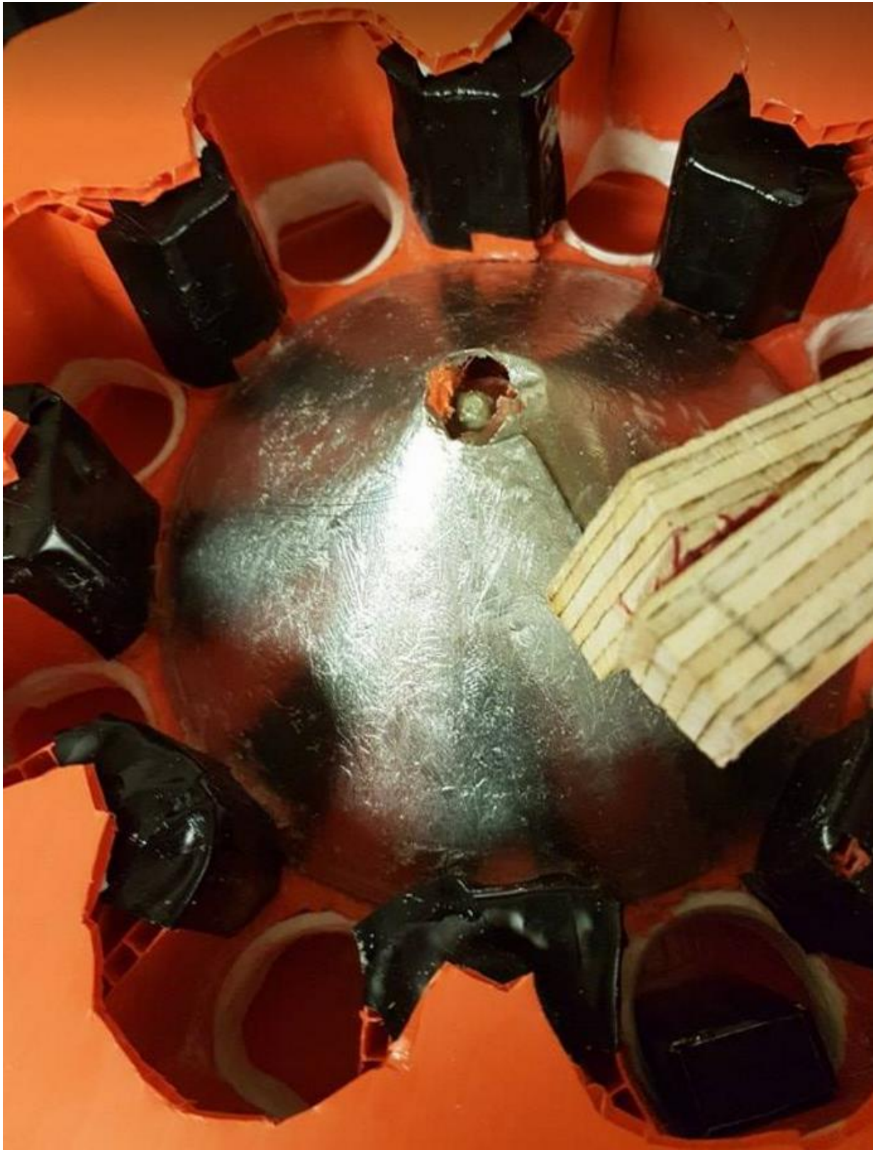
Figure 10.1.2.1.5 Top view of rate limiter showing the dome and the holes for the batteries
