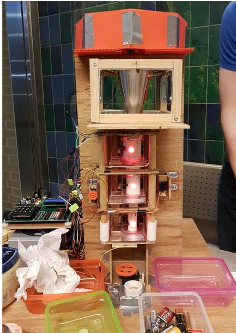
Figure 14.1.2 Front view of main machine. Rate limiter, funnel, block system + electrode tower, ramp + bins
