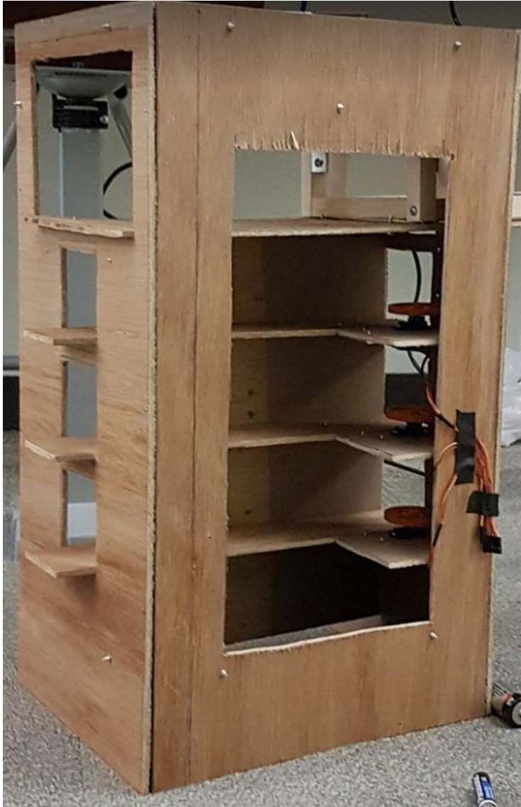
Figure 10.1.2.8.1 Platform that supports rate limiter, circuitry, and battery blocks
