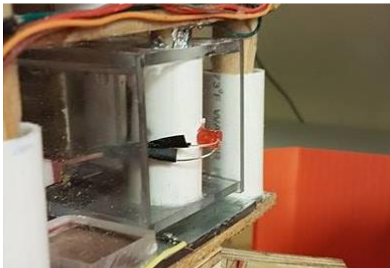
Figure 14.4.6 Image of electrode tower lowered into AA block
