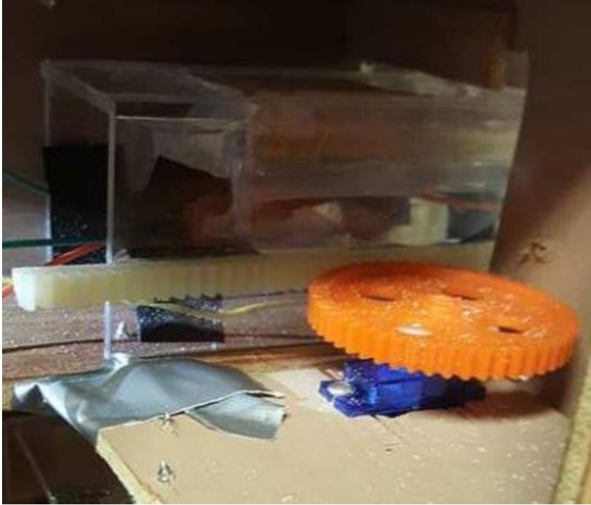
Figure 10.1.2.3.3 Rack and pinion mechanism for the C battery block
