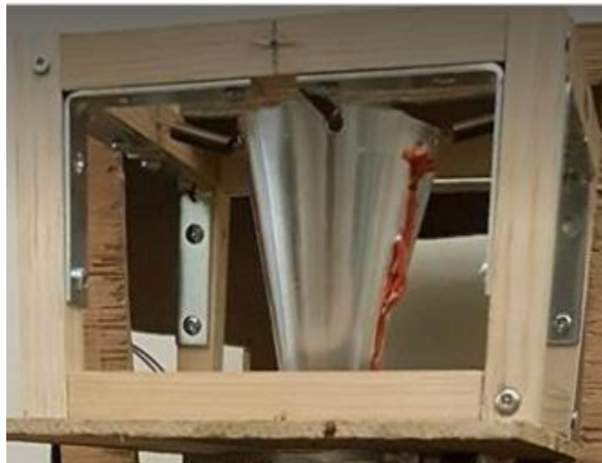
Figure 10.1.2.2.6 Front view of wooden rectangular prism that supports the funnel
