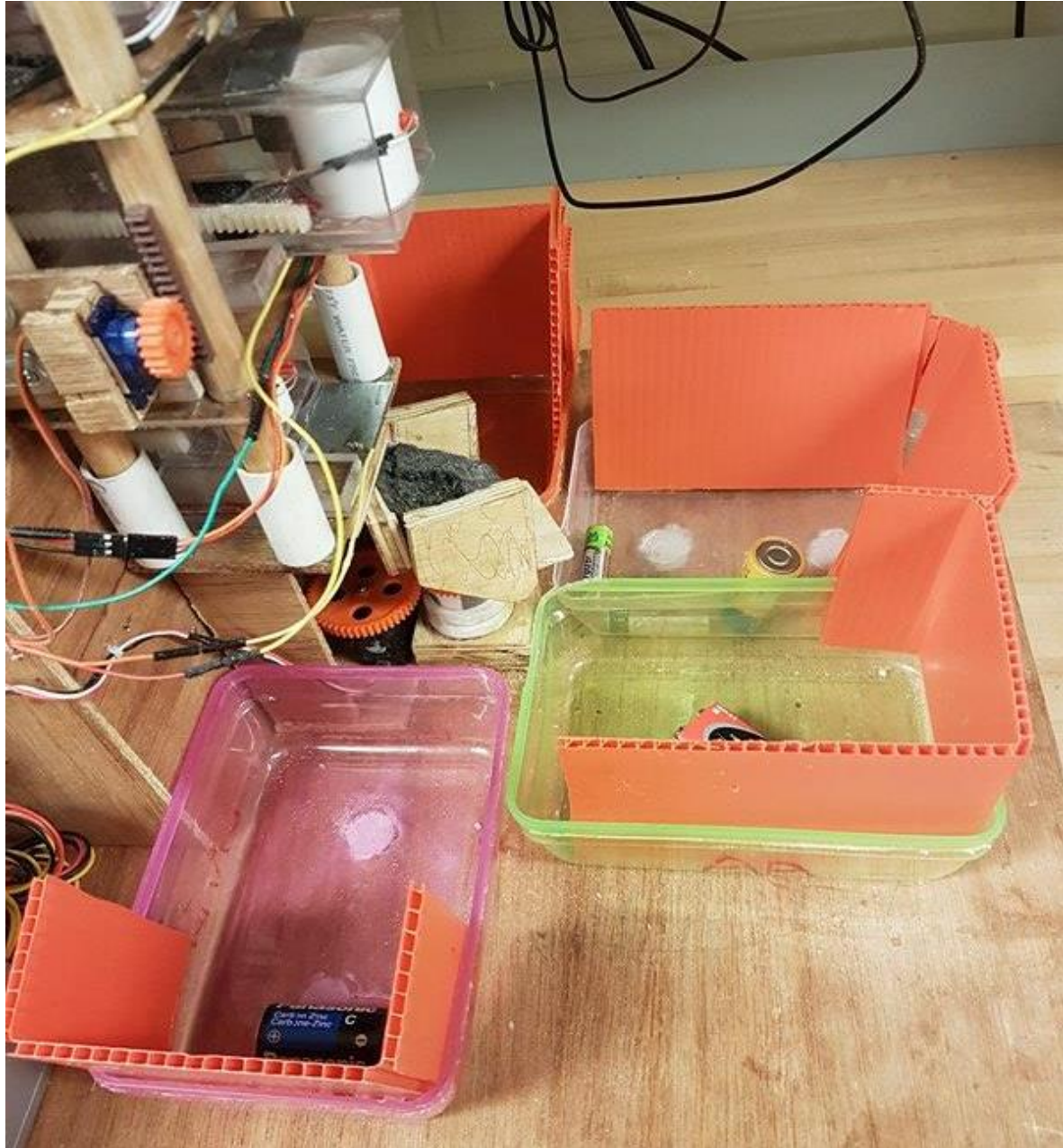
Figure 14.5.1 View of the ramp system with the C block extended. A battery in the C block would fall down onto the ramp and land in the bin it is pointing to.
