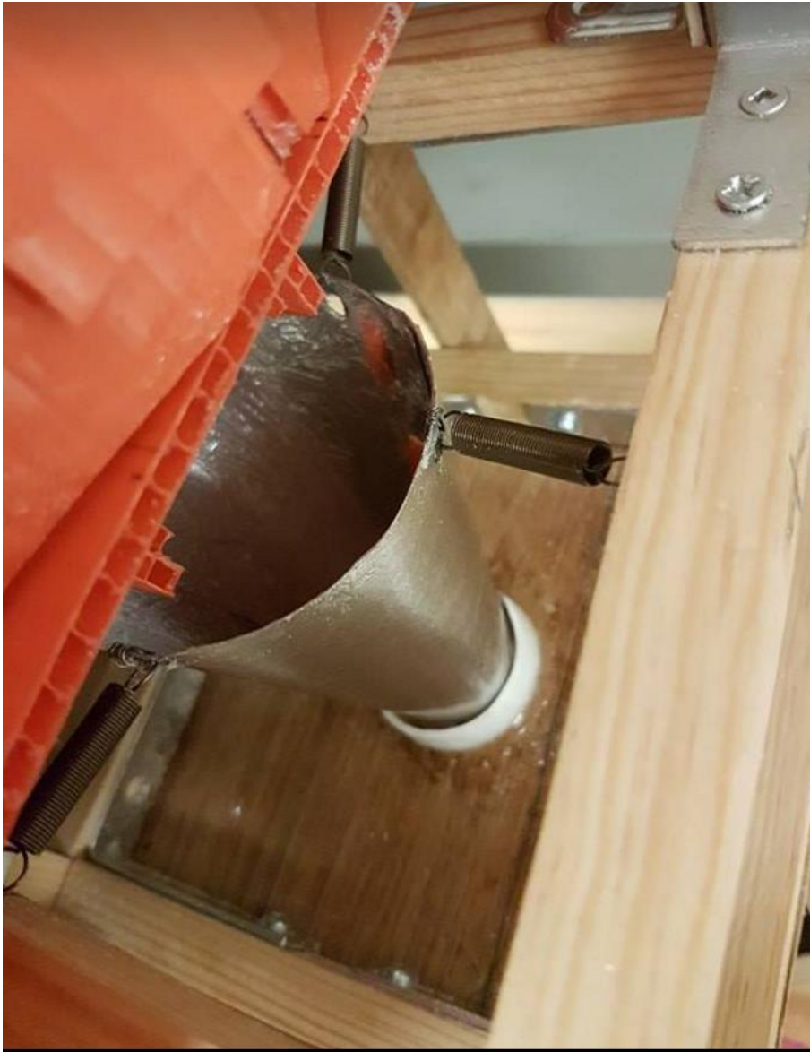
Figure 10.1.2.2.2 Isometric view of funnel and springs. It is positioned right beneath the rate limiter (orange corrugated plastic)
